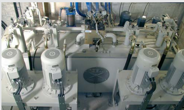
Hydraulikaggregate - Hydraulic Power Units
