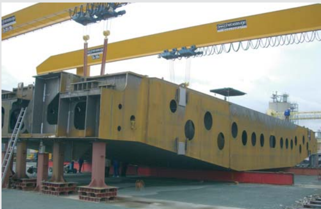
Fertigung Torsegmente - Manufacturing Gatesection
