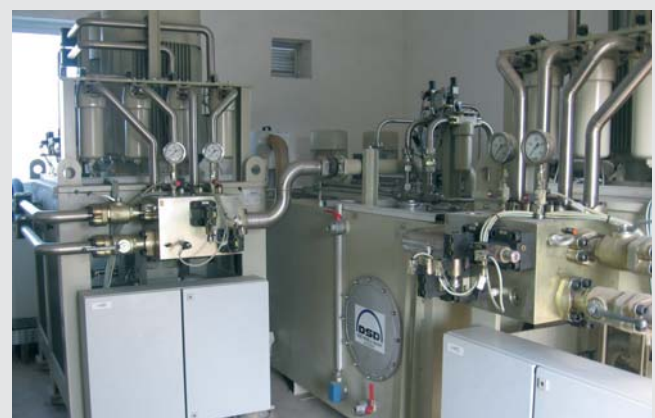
Hydraulikaggregate - Hydraulic Power Units
